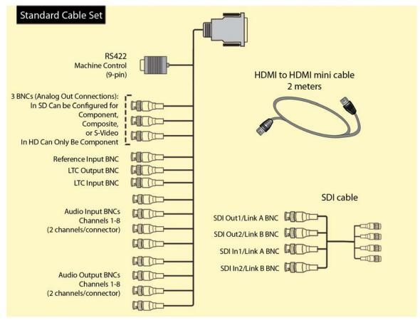
The KONA LHi and LHe Plus cards use the breakout cable shown below providing XLR balanced audio connectors, an RS-422 9-pin connector, and BNCs for video I/O and reference connection.
