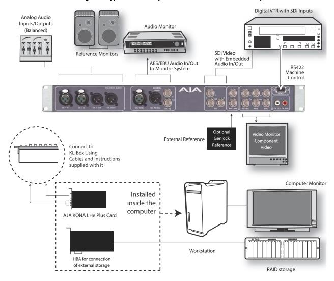
Figure 9. Typical LHe Plus System Connections—Shown with Optional KL-Box
