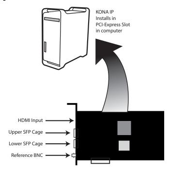
The KONA IP card fits into a standard PCle slot of a computer or into PCle chassis. The end spine has a full size HDMI output connector, two SFP cages (Upper and Lower), and a reference BNC connector.
