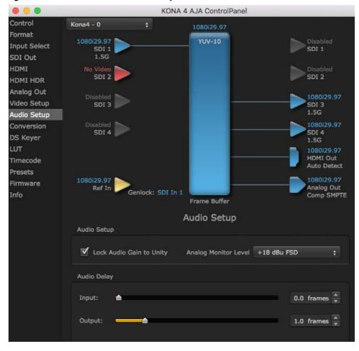
Figure 20. AJA Control Panel, Audio Setup Screen
