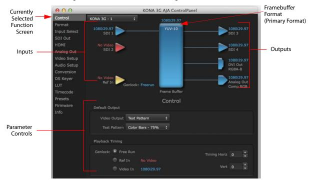
Figure 1. AJA Control Panel, Block Diagram and Controls
