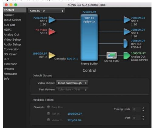
Figure 6. AJA Control Panel, Control Screen
