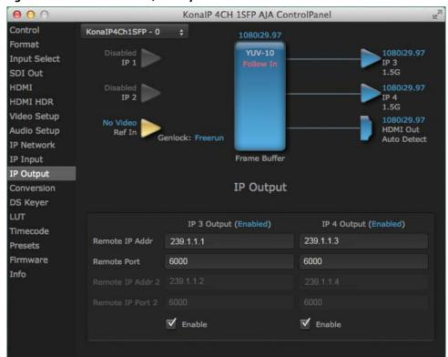
**NOTE:** The IP Output 3 and IP Output 4 labels do not represent the physical SFP cages on the KONA IP. They represent different transmissions being sent by the KONA IP card, possibly over the same 10GbE link.
