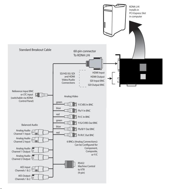
**Typical System** Figure 11 on page 32 shows typical system interconnections for a system with digital A/V sources. Your system may differ depending on VTRs, audio monitoring, and video monitoring.
