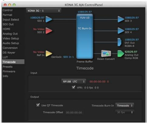
Figure 28. AJA Control Panel, Timecode Screen
