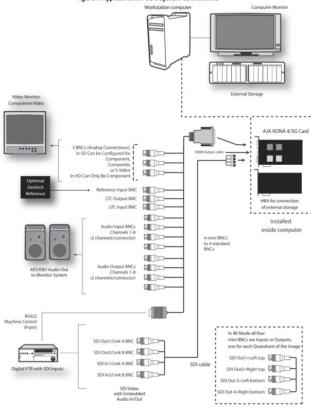
Figure 7. Typical KONA 4/3G System Connections
